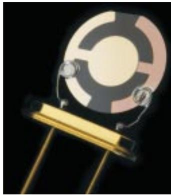
Using targeted antibodies, the quartz microphone could be fashioned to recognize the sounds of a multitude of viruses. “It could even detect bioterrorist germs,” Cooper says: add a microthin film of an-
